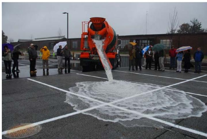
**A demonstration showing how quickly pervious pavement can handle flow. This pervious concrete drained 2,000 gallons of water in less than 3 minutes with no runoff. (Photo: US EPA, 2010)**
