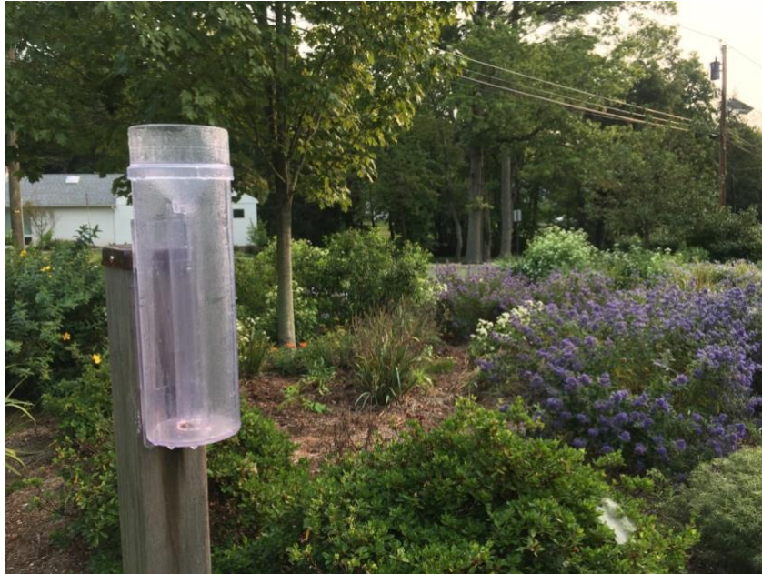
Figure 3. A CoCoRaHS rain gauge used by community scientists to watch and report weather conditions.
